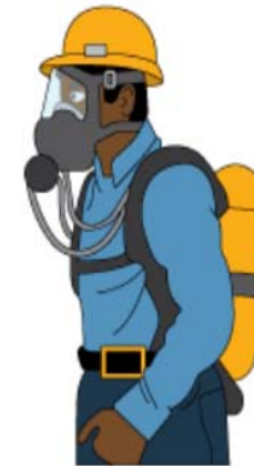
Full Facepiece Self-Contained Breathing Apparatus (SCBA) Pressure demand mode is APF=10,000 Needs to be fit tested
