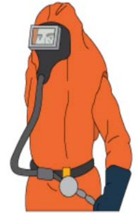
Full Facepiece Abrasive Blasting Continuous Flow APF=1,000 Needs to be fit tested
