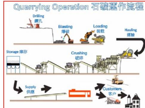
Aggregate comes from quarrying. Quarrying is a process of extracting rock from the hill through drilling and blasting operation then load to lorry and transport to the crushing plant to fragment and screen to different size then sell to customers.
