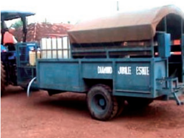
Figure 5: Improved trailer to minimize the risk of chemical exposures – trailer for spraying activities
